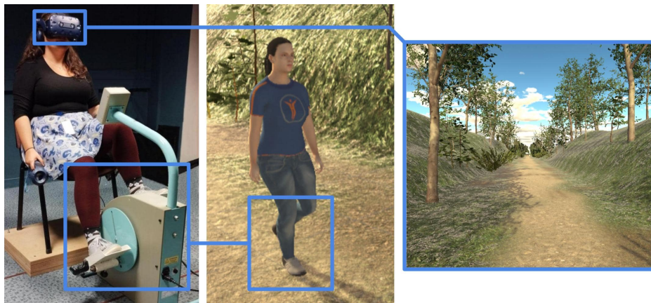
Fig. 1: We introduce assisted motion to walking-by-cycling using a motorized bike (left). The user embodies an avatar which is viewed in first-person perspective (right). The bike drives the user’s legs in a cycling motion, which makes the avatar walk in synchrony (middle) without requiring effort from the user.
