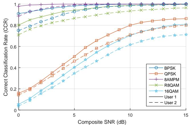
Fig. 11. Correct Classification Rate (CCR) for both signals in the context of two overlapping signals – SIR  $\in [0; 6]$  dB – Blind scenario –  $N = 1e^4$
