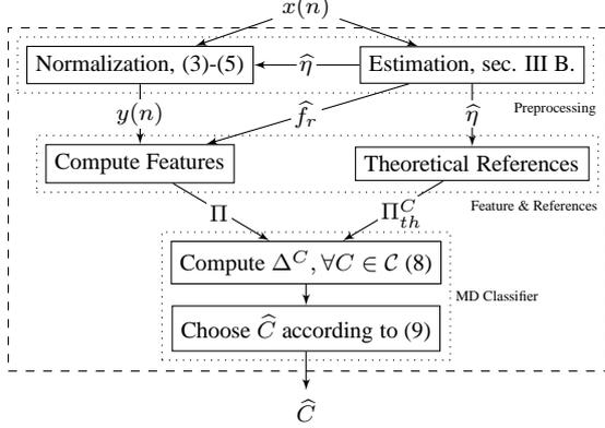
Fig. 3. The proposed fully-blind AMC algorithm
