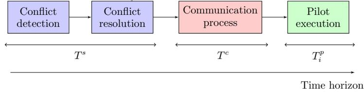
Figure 2: Structure of the maneuver delay
